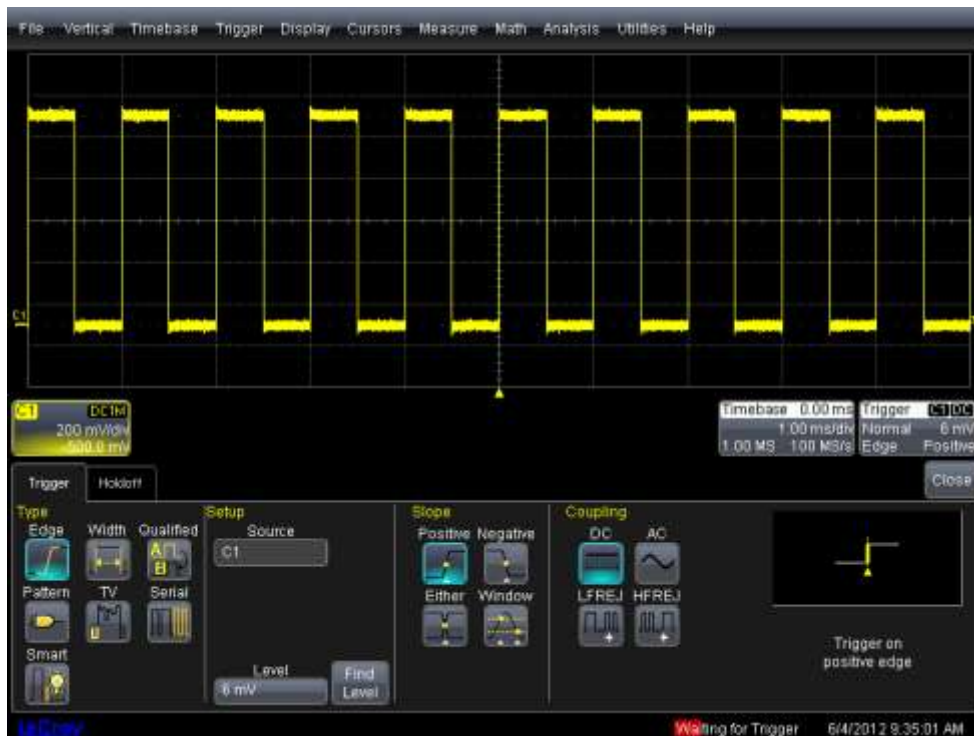
Figure 8 - The "Waiting for Trigger" message indicating the scope in not triggering
