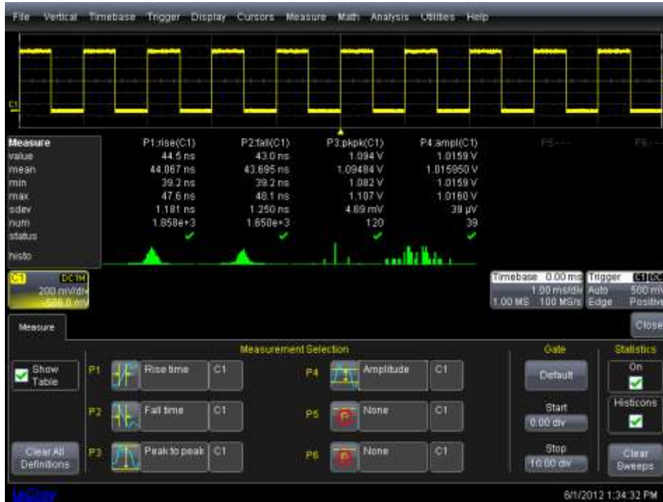
Figure 10 - Parameter measurements with statistics and histicons.
