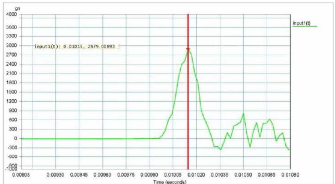
Figure 13: Shock (g-force) as a function of time showing 3000 g pulse.
