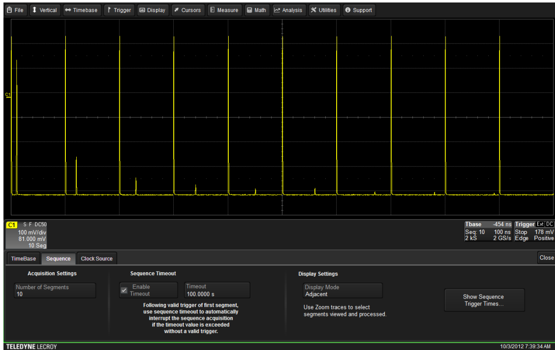
Figure 2: Upon invoking the Sequence Mode option in the Timebase tab, users are presented with the controls dialog at the bottom of the screen
